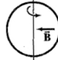
(e) Rotating the loop by pulling the left side toward us and pushing the right side in; the magnetic field points from right to left
