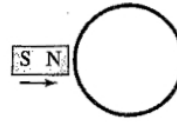
(d) N magnetic pole moving toward the loop in the plane of the page
